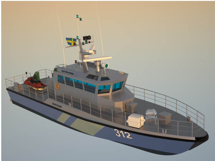
Figure 8: Projected new coast guard craft with composite material hull.
