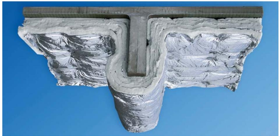
This CSC deck section shows the fire insulation in place
